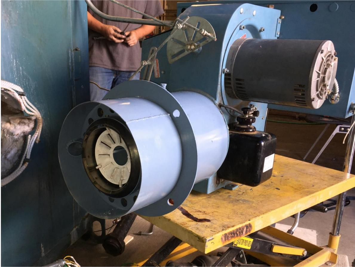
**Figure 1 - The newly refabricated cylindrical section of the power burner that is inserted into the boiler. The end that is designed to induce the complete combustion of fuel has been restored.**
