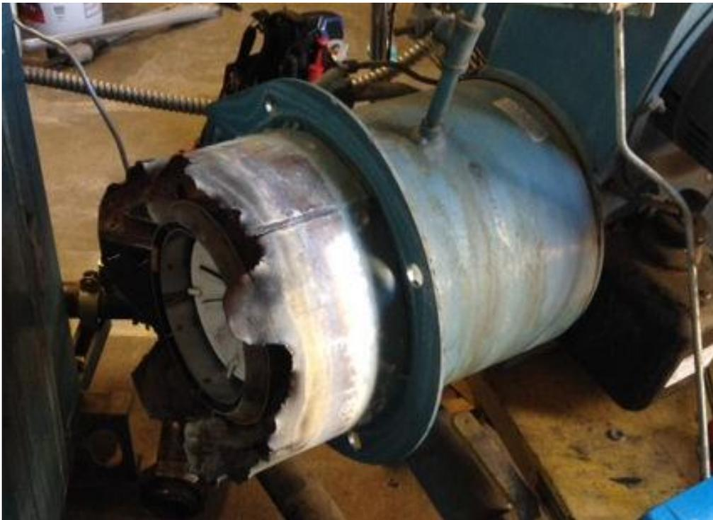
**Figure 2 - The cylindrical section of the power burner that is inserted into the boiler. The end that is designed to induce the complete combustion of fuel is completely burned away.**
